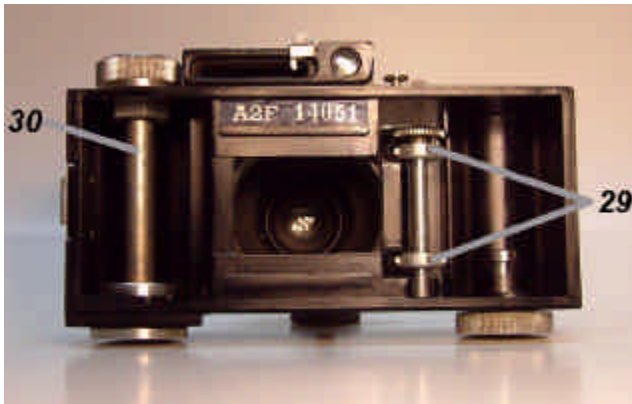
Fig. 4-6: Inside view of an Argus A2F
